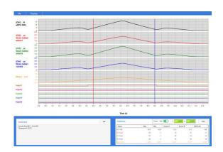
Statistical values such as max. and min. values automatically displayed after recording. The measurement values checked for each graph at any stage.
