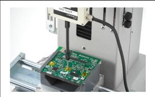
A switch on the board is pressed at a constant force, and the deformation (deflection) of the entire board and localized strain (3 locations) are measured.
