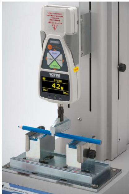
Specify the necessary parameters according to each test method, automatically calculate the "bending stress", and display the measurement results. Dedicated report templates and CSV formats are available to output bending stress and related parameters.
