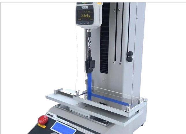
The measurement results are automatically converted and displayed in the set peel force unit (N/10mm, etc.) by advanced setting conditions such as sample width, conversion unit, and calculation interval. It also displays the result of standard conformity judgment of selected data.
