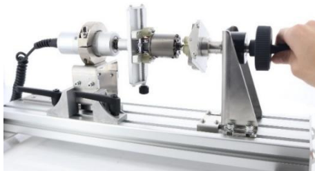
Torque measurement of a small motor
