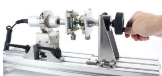
Torque measurement of a volume switch
