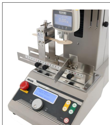
CBJ-200N Testing Image (Cantilever bending test of cutlery)
