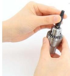
A photograph showing a person's hands holding a small, round sample and inserting it into the open jaws of the Jacobs Chuck GC-5/15. |
