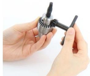
A photograph showing a person's hands using a black handle to close the jaws of the Jacobs Chuck GC-5/15, securing the sample. |
