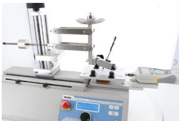
COF test of a pen using VWF-10N-J*
