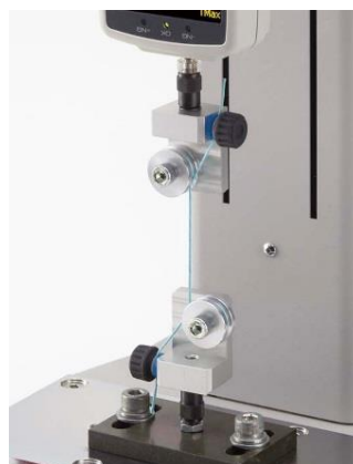
Test Image (Tensile test of fiber)
